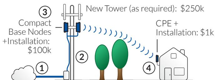
Deployment of elements 3 and 4 is very straightforward. A tower can be outfitted with BNs in 2 or 3 days of on-site work, with a total cost of hardware, BNs, and labor on the order of \$100k per tower. The installation of the RN at the home is typically a couple of person-hours – with most of that time spent running an Ethernet cable from the outdoor unit into the home. RN hardware and installation are typically in the range of \$1k.
