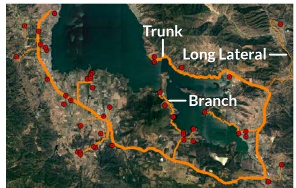
Adding measurements of all the fiber elements and applying an industry benchmark for rural trenching costs per mile yields a total cost for the trenching in this project of \$6.8M, or \$120k per location. Trenching alone for the all-fiber approach is more than 40x the cost of the complete DigitalPath deployment.
