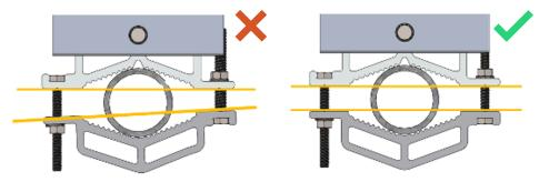
6. With the clamp in the final position, torque 4 bolts with incremental steps at approximately 40%, 70%, and 100% of full torque rating while ensuring the brackets stay parallel.
