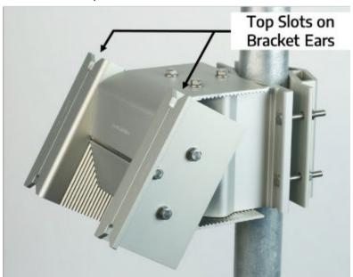
2. Slide the base node into the top slots in the bracket ears using the partially-installed bolts from Step 1. Make sure that the wedge lock washers are on the outside of the bracket and not between the base node and the bracket.
