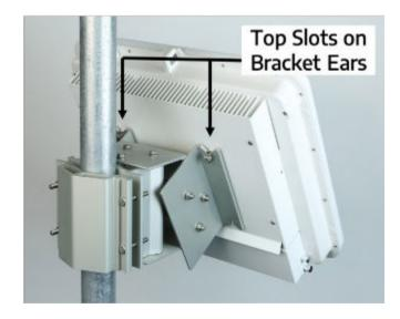
3. Install 2 M8 x 25 mm bolts with wedge lock washers in the two remaining lower slots on the bracket ears. Make sure that the wedge lock washers are on the outside of the bracket and not between the base node and the bracket.
