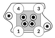
The G1 base node has a four-pin power interface that accepts the Harting push-pull power connector.
