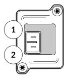
The G2 base node power port has a two-pin interface that accepts the OCTIS power connector.
