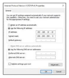
3. The MGMT port has a default IP of 192.168.10.2/24 with no VLAN. Enter this address into a web browser to access the base node's web interface. Google Chrome is the supported browser.
